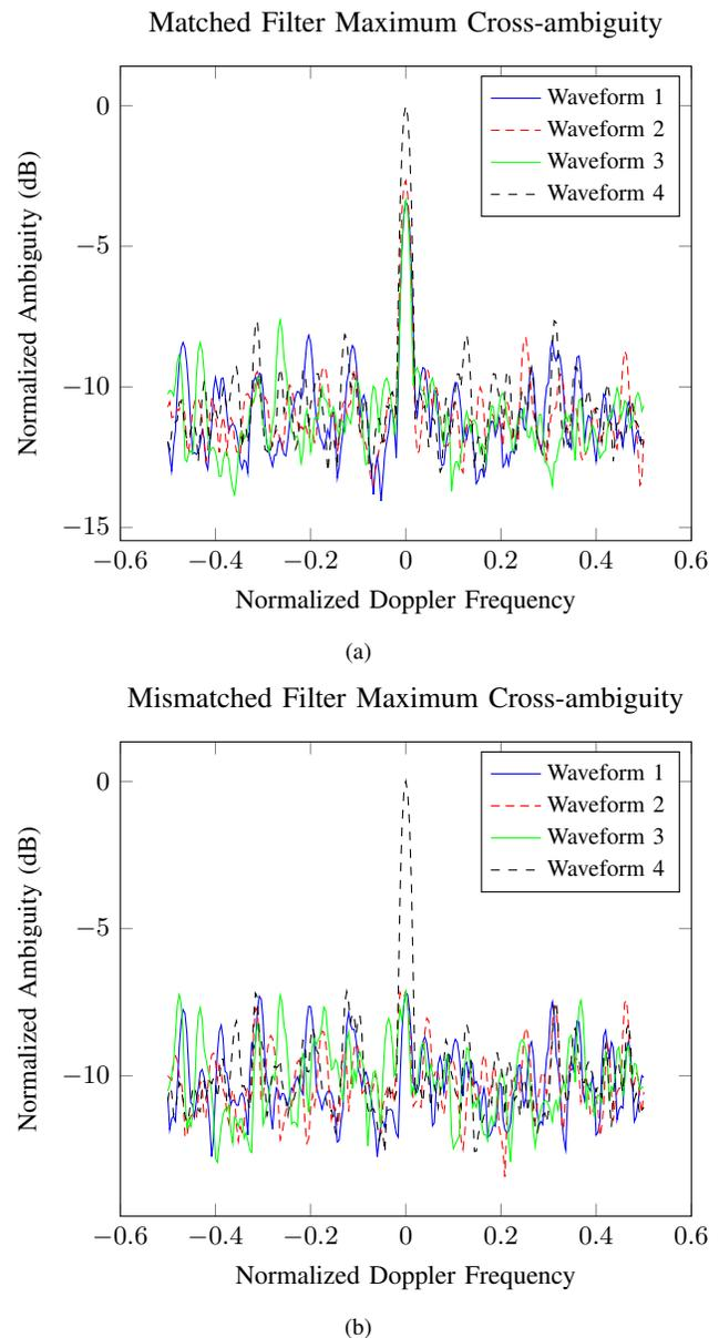
Fig. 4. Maximum cross-ambiguity of the waveform set with high cross-correlation for (a) matched filter and (b) the mismatched filter for the fourth waveform. The mismatched filter does not have the cross-correlation peaks at zero Doppler that the matched filter has.
