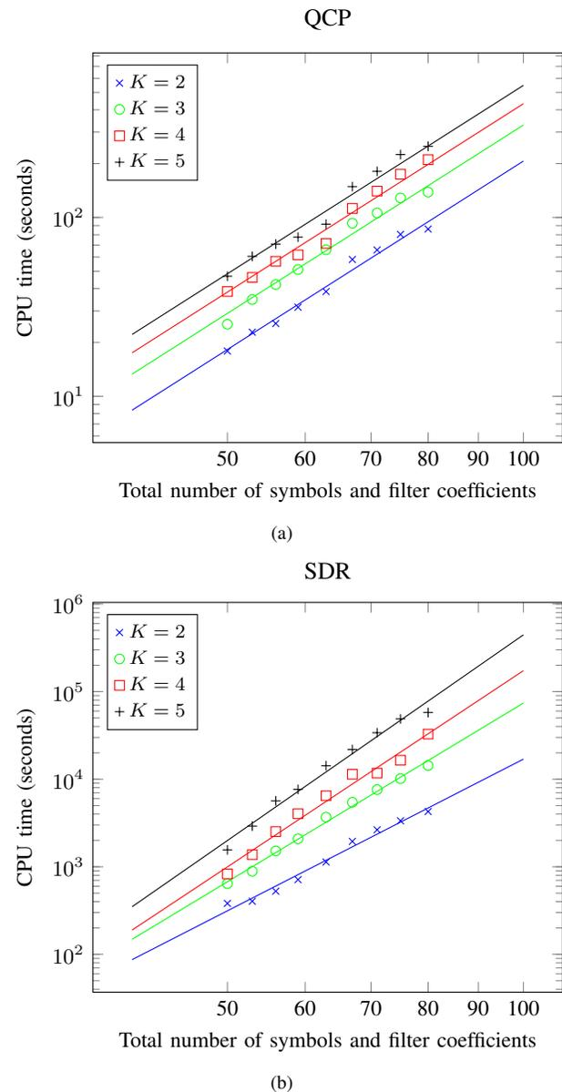
Fig. 8. The CPU time needed for optimizing the mismatched filter using (a) QCP approximation or (b) SDR formulation. The number of waveforms is  $K$ . The QCP approximation is computationally much less complex than the SDR formulation of the problem.
