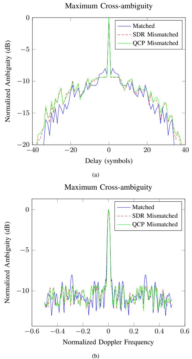
Fig. 2. Maximum cross-ambiguity of the waveform two of [5] and the receiver filters over (a) the Doppler frequency and (b) the delay. Lower sidelobes are achieved with the mismatched filters. The difference between the SDR and the approximate QCP filters is small.
