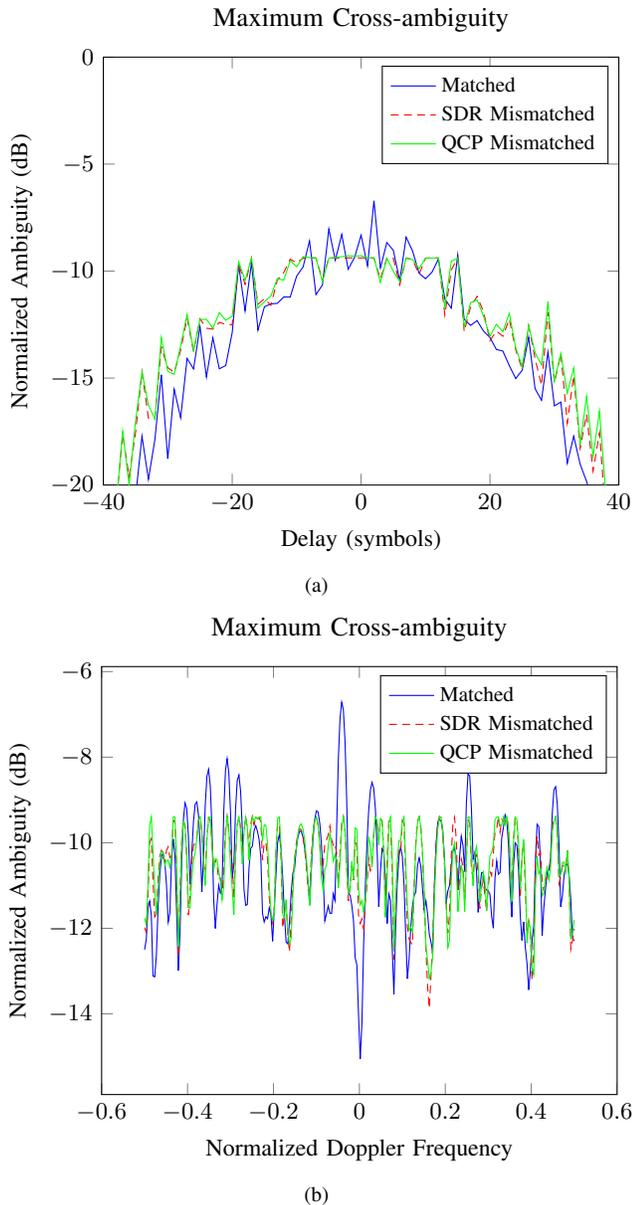
Fig. 3. Maximum cross-ambiguity of the waveform number four in [5] and the receiver filters for waveform two over (a) the Doppler frequency and (b) the delay. Considerably lower peak cross-correlation is achieved with the mismatched filters. Again, the difference between the SDR and the approximate QCP filters is small.
