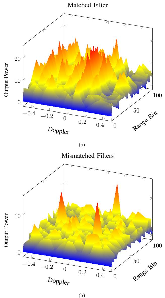
Fig. 6. Range–Doppler plots for (a) matched filter and (b) mismatched filters. The targets are buried in the interference when the matched filter is used but are clearly distinguishable with the mismatched filter.
