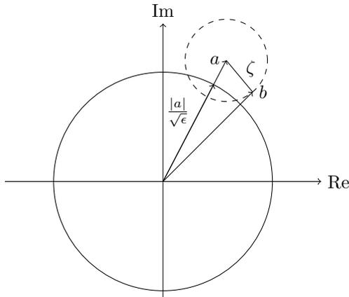
Fig. 1. Constraining the signal loss. For the signal loss to be less than  $\epsilon$ , the filter response  $b$  needs to be outside the solid circle. This is achieved by constraining  $b$  to be inside the dashed circle and setting the radius  $\zeta$  so that the dashed circle lies outside of the solid circle.
