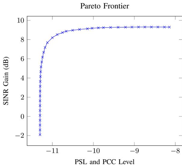
Fig. 5. Pareto frontier of the mismatched filter design showing the best achievable combinations of the SINR gain and minimum PSL and PCC. Filters with excellent trade-off between PSL and PCC level and SINR gain can be achieved along the Pareto curve.
