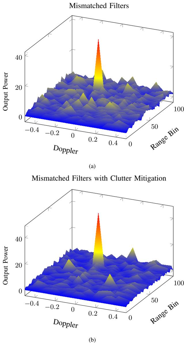
Fig. 7. Range–Doppler plots for (a) mismatched filters with interference mitigation and (b) mismatched filters with combined interference and clutter mitigation. Without the clutter mitigation, it is difficult to detect the targets in (a) because of the sidelobes. With the clutter mitigation in (b), targets are clearly visible.
