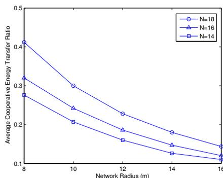
Fig. 11: Average cooperative energy transfer ratio vs. network radius.
