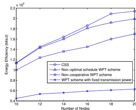
Fig. 10: Energy efficiency vs. number of nodes.
