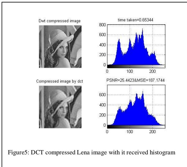
Figure5: DCT compressed Lena image with it received histogram
