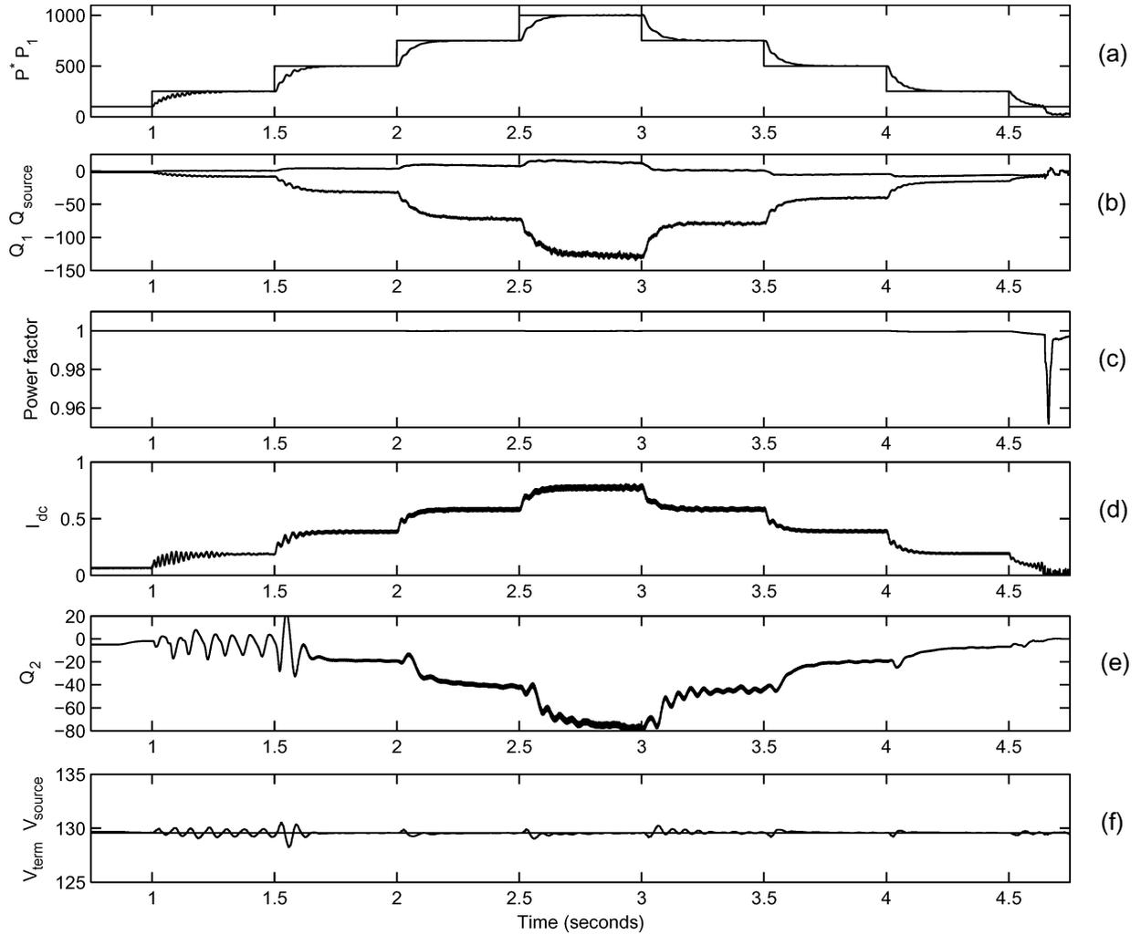
Fig. 10. Reactive power responses under power factor and terminal voltage control for a series of step changes to real power.
