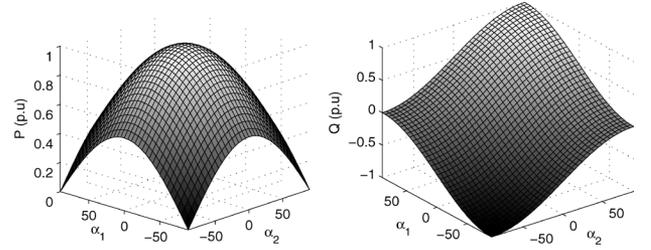
Fig. 4. Calculated real and reactive power for varied firing angle ( $\pm 90^\circ$ ).
