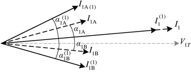
Fig. 3. Firing shift control maintaining constant reactive power at the sending end for two different system strengths.
