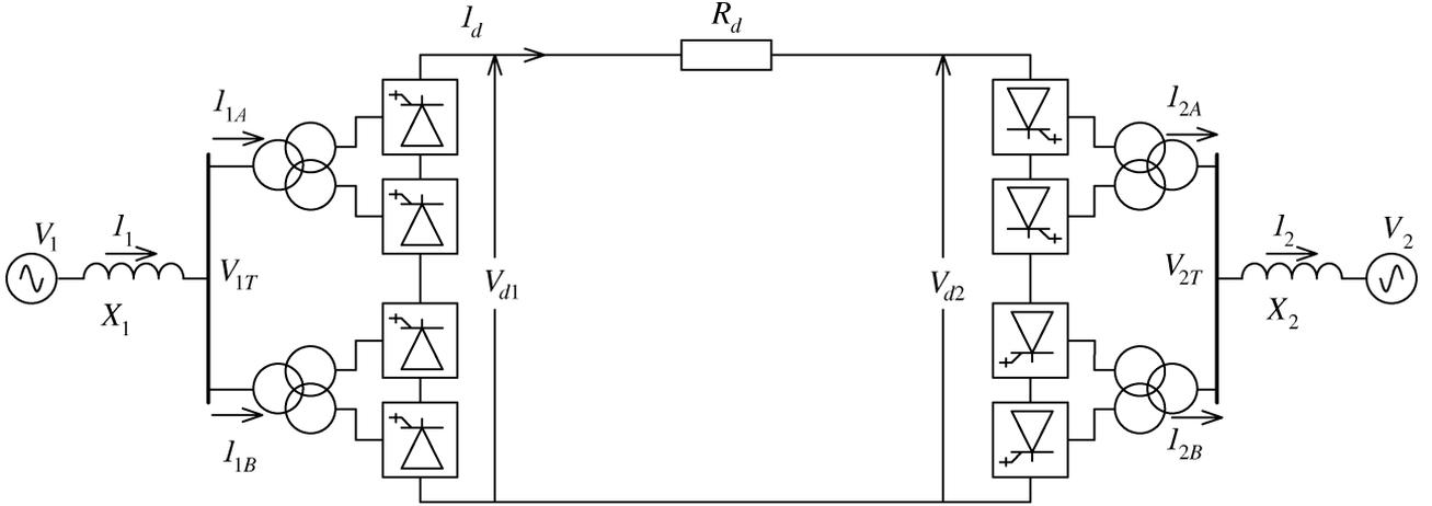
Fig. 1. Simplified diagram of a dc link connecting two ac systems.
