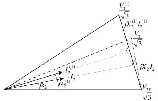
Fig. 2. Operating conditions at the receiving end for two different system strengths.
