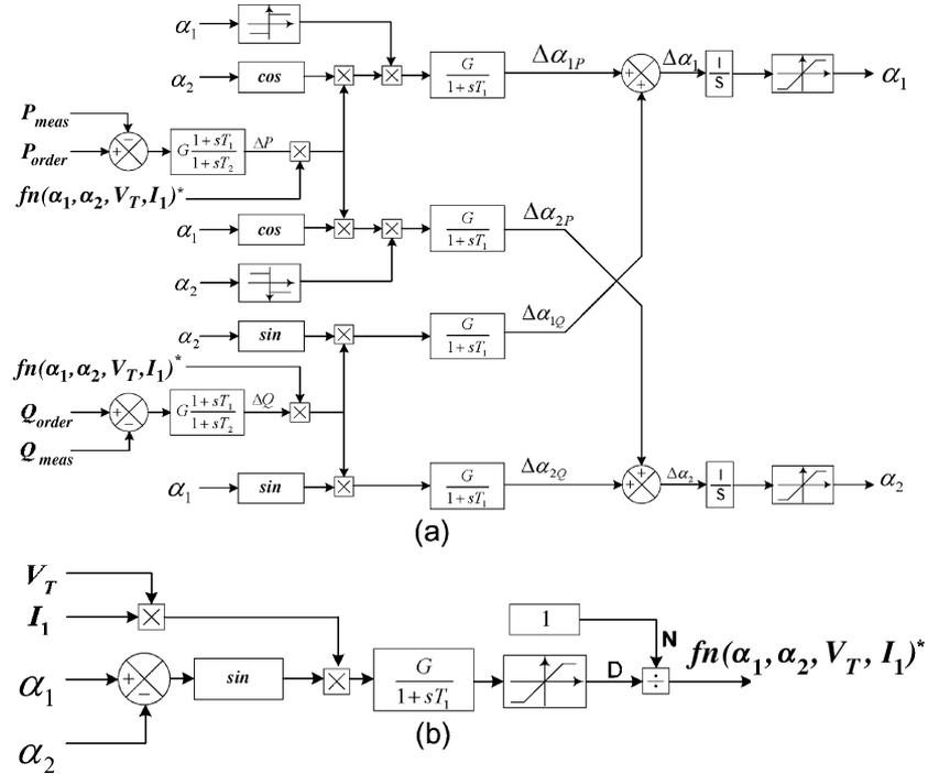
Fig. 8. Sending end controller block diagram, with the main linearizing components in (a) and the common angle difference calculation in (b).
