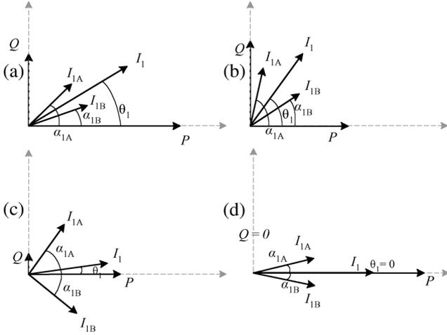
Fig. 5. Firing shift control providing (a) large  $P$  and  $Q$ , (b) large  $Q$  and smaller  $P$ , (c) small  $P$  and  $Q$ , and (d) large  $P$ , no  $Q$ .
