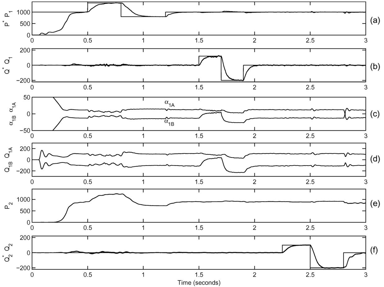
Fig. 9. Real and reactive power order changes at the sending and receiving ends.
