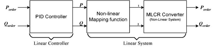
Fig. 6. Block diagram of the nonlinear system control objective.
