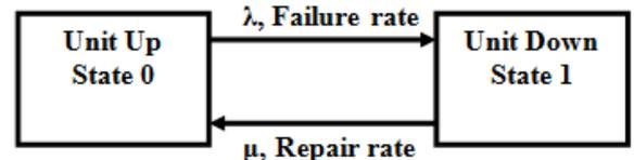
Fig. 4. A two-state model for the generating unit [2, 3]
