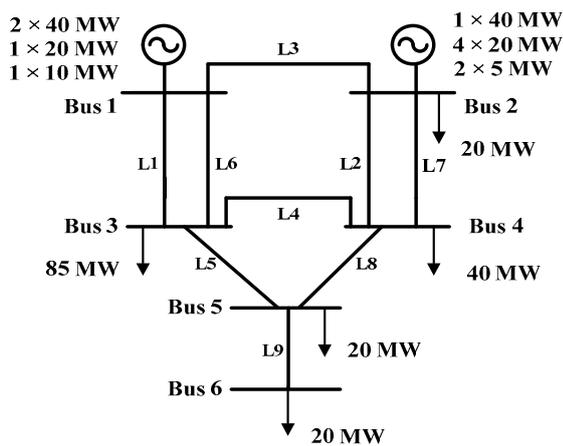
Fig. 7 Single line diagram of the Roy Billinton Test System (RBTS) [15]
