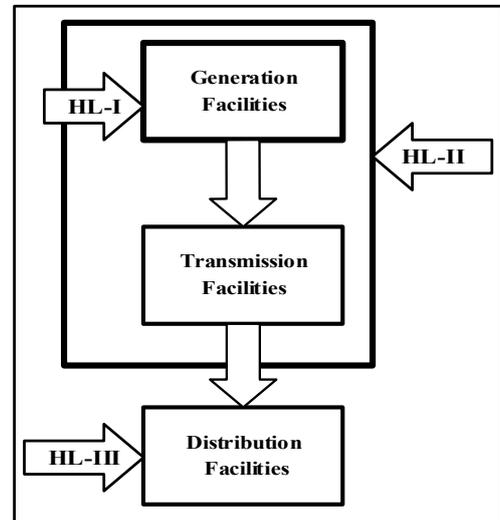
Fig. 2. The hierarchical levels of a power system [2, 3].
