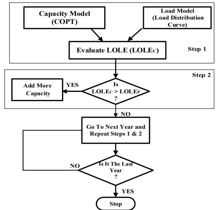
Fig. 5. Flow chart for the adequacy evaluation using the loss of load method [18]
