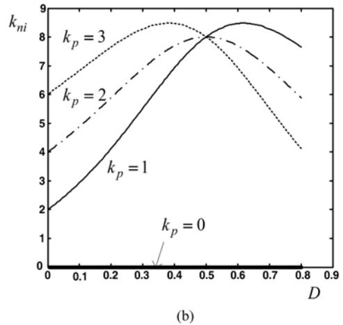
Fig. 6. Theoretical stability boundaries of  $k_{ni}$  as a function of  $D$ . (a)  $S_r = \frac{1.0D}{1-D}$ . (b)  $S_r = \frac{2D}{1-D}$ .
