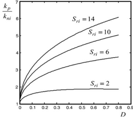
Fig. 7. PI gain curve for the critically damped response.
