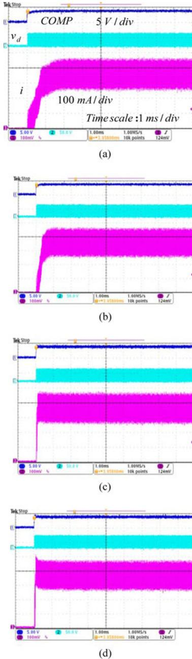
Fig. 12. Start-up transient responses with increasing integral gain  $k_{ni}$  ( $V_i = 40$  V,  $V_o \approx 16.25$  V,  $k_p = 0.84$ ,  $R'_1 = 4.2$  k,  $R'_2 = 12$  k). (a)  $k_{ni} = 0.02$  ( $C'_1 = 0.1$   $\mu$ f). (b)  $k_{ni} = 0.1$  ( $C'_1 = 20$  nF). (c)  $k_{ni} = 0.29$  ( $C'_1 = 6.8$  nF). (d)  $k_{ni} = 0.38$  ( $C'_1 = 5.3$  nF).
