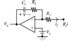
Fig. 3. PI error amplifier circuit.
