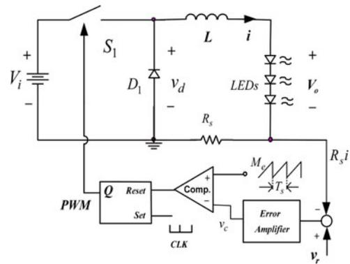
Fig. 1. Duty-cycle-controlled buck LED driver with constant-frequency controller.
