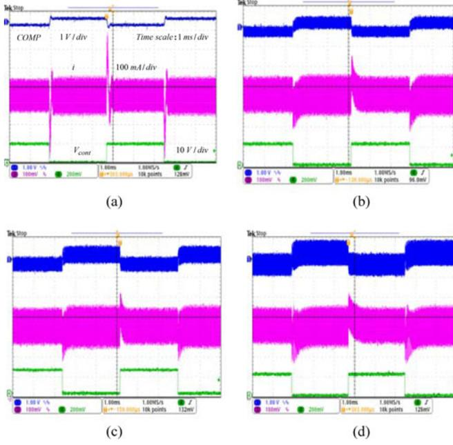
Fig. 10. Transient responses for step load change between 3 and 5 LEDs ( $V_i = 40$  V,  $k_{ni} = 0.2$ ,  $R'_2 = 12$  k,  $C'_1 = 10$  nF). (a)  $k_p = 0.1$  ( $R'_1 = 0.5$  k). (b)  $k_p = 0.84$  ( $R'_1 = 4.2$  k). (c)  $k_p = 1.3$  ( $R'_1 = 6.5$  k). (d)  $k_p = 2.0$  ( $R'_1 = 10$  k).
