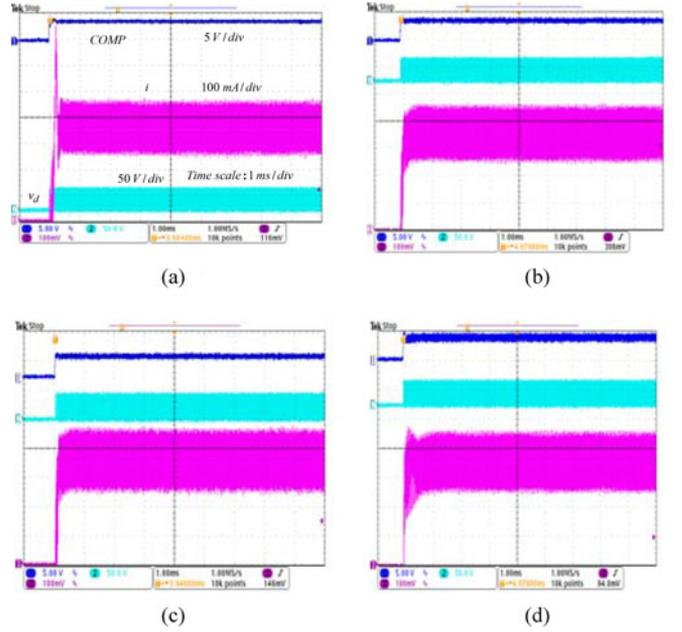
Fig. 9. Start-up transient responses with increasing proportional gain  $k_p$  ( $V_i = 40$  V,  $V_o \approx 16.25$  V,  $k_{ni} = 0.2$ ,  $R'_2 = 12$  k,  $C'_1 = 10$  nF). (a)  $k_p = 0.1$  ( $R'_1 = 0.5$  k). (b)  $k_p = 0.84$  ( $R'_1 = 4.2$  k). (c)  $k_p = 1.3$  ( $R'_1 = 6.5$  k). (d)  $k_p = 2.0$  ( $R'_1 = 10$  k).
