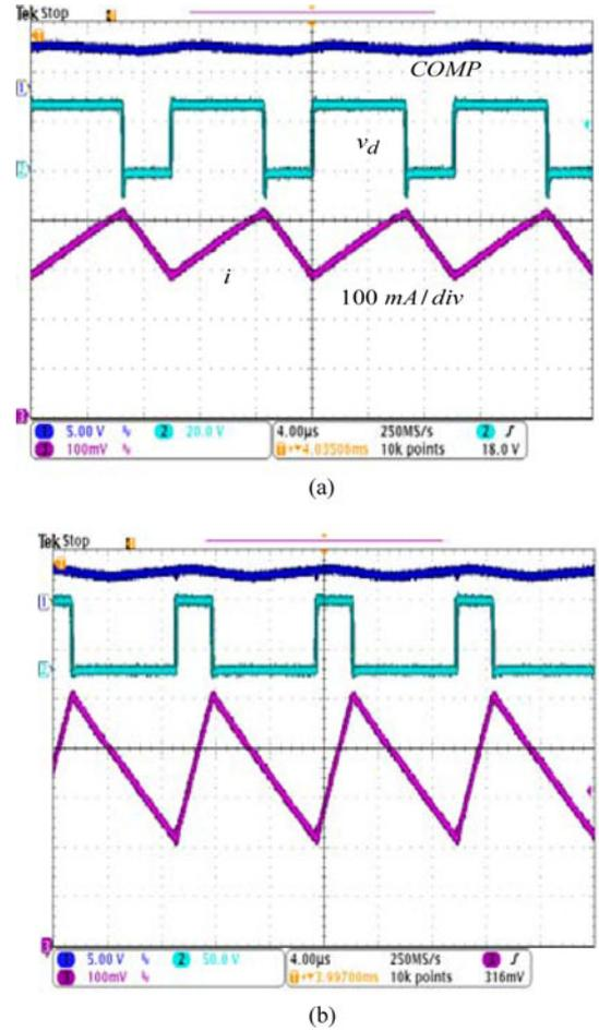
Fig. 13. Steady-state waveforms with increasing the input voltage ( $V_o \approx 16.25$  V,  $k_p = 0.84$ ,  $k_{ni} = 0.2$ ). (a)  $V_i = 27$  V. (b)  $V_i = 70$  V.
