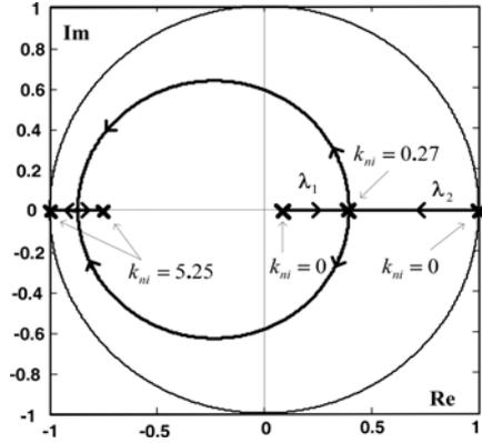
Fig. 5. Root locus as a function of the I gain  $k_{ni}$  ( $k_p = 0.84$ ,  $D = 0.4$ ,  $S_r = \frac{1.5D}{1-D} = 1.0$ ).
