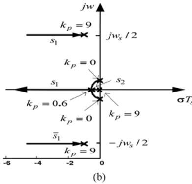
Fig. 4. Root locus as a function of the P gain  $k_p$ : (a) in the  $z$ -plane and (b) in the  $s$ -plane ( $k_{ni} = 0.2$ ,  $D = 0.45$ ,  $S_r = \frac{1.0D}{1-D} = 0.82$ ).
