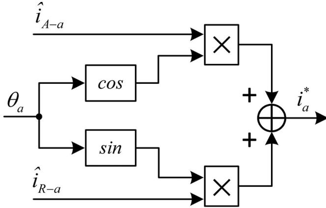
Fig. 3. Current reference generation for phase  $a$ .
