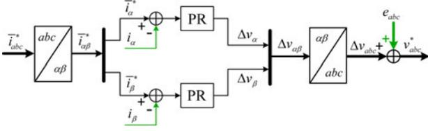
Fig. 5. Current control loop with PR controllers.
