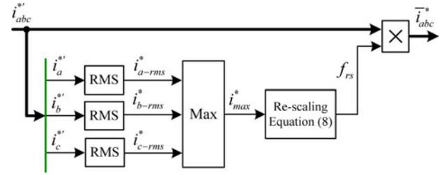
Fig. 4. Control diagram for rescaling the current references to avoid overcurrents.
