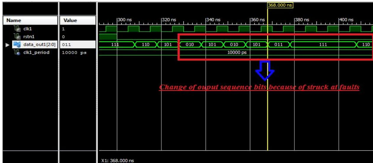
Figure 6(b): Simulation of BIST Architecture with Fault
