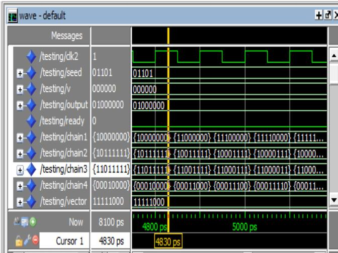
Fig. 8. Testing of Multiplier using Reconfigurable Johnson counter and LFSR
