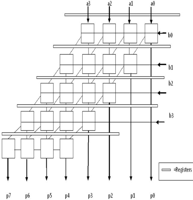
Figure 2. Braun array multiplier
