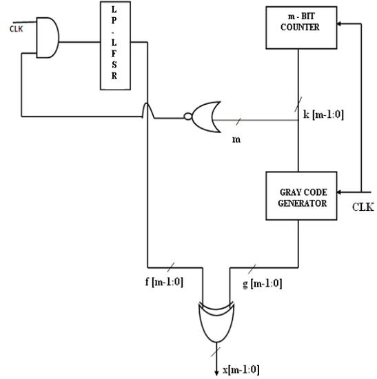
Figure 3. Low Power Test Pattern Generator
