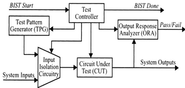
Figure 1. BIST Basic block diagram
